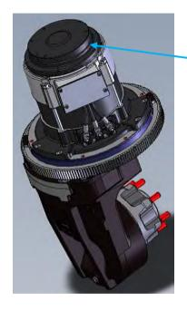
Front wheel drive parking brake can only be unlocked electrically (with tool kit 01381500)
