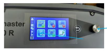
"Rotate" until the information field is framed in yellow confirm by "Pressing" rotary push button
